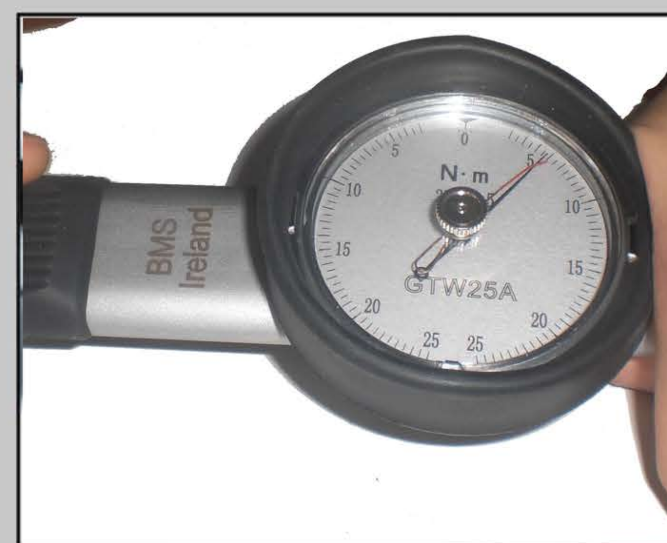
Model: GTW25 Metric Reading: 5.5Nm
